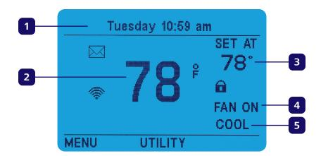
1 Messaging Area Displays day and time, thermostat, and Delmarva Power-related messages. In the event of a power outage, the clock will maintain the correct time for 48 hours
